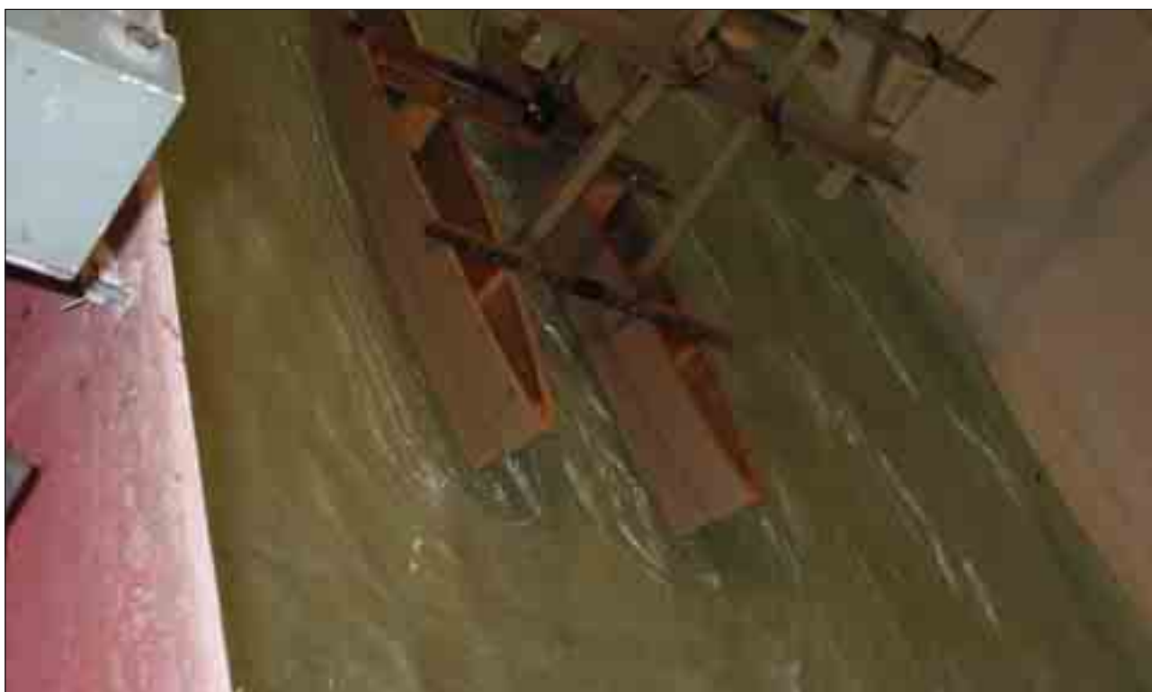
Tank tests were undertaken to develop the optimum low 'wash' hull design
