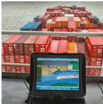
INTRODUCED PORTABLE PILOT UNITS, WHICH BRING TOGETHER ELECTRONIC CHARTS, OTHER SAFETY AND NAVIGATION INFORMATION, WITH PRECISE, REAL TIME POSITIONING DATA, TO ASSIST PILOTS BRINGING LARGE SHIPS ON TO THE THAMES
