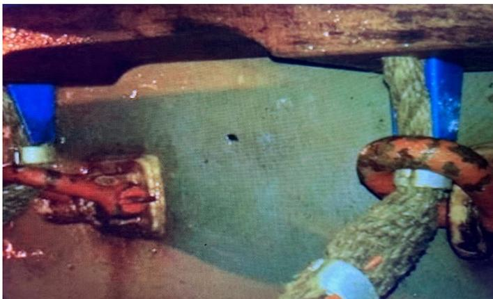
*Image showing stress caused on chocks and steps*
